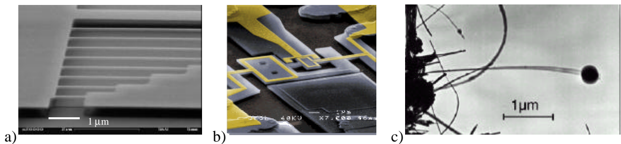
Fig. 1. State of the art NEMS. a) 50 nm-wide Si beams resonating at 10-400 MHz (Carr, Evoy, et al , Cornell Univ. [1]). b) Nanofabricated paddle as ultrasensitive electrometer (Roukes et al , Cal Tech [3]) c) Carbon nanotube (1-5 MHz range resonances) as a ultrasensitive nanobalance (De Heer et al. , Ga Tech [4])
