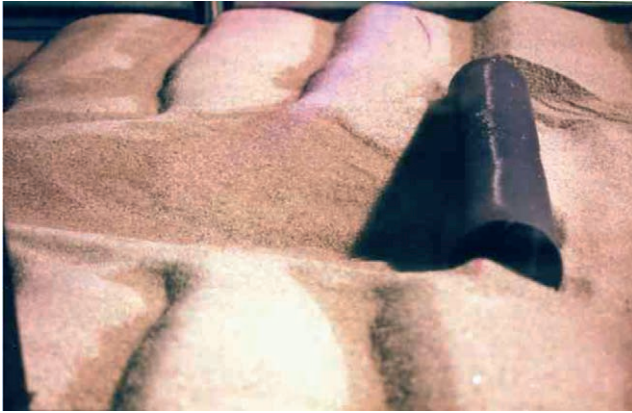
Fig. 8. A photograph showing an oblique view of the expanded scour pattern (regime III) around a cylinder. The onshore direction is to the left. Time t = 78 min after the initiation of wave forcing. Experimental parameters: D = 8 cm, \omega = 0.4 Hz, \varepsilon = 11.7 cm, U = 45.7 cm s -1 , KC = 10 , Sh = 0.27 .
