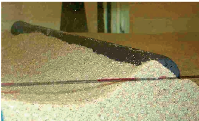
Fig. 6. An example showing typical scour pattern surrounding a long cylinder. Experimental parameters: D = 4 cm, KC = 20 , Sh = 0.07 , sand accumulation can be seen on the onshore side of the cylinder. Time t = 320 min. The onshore direction is to the left. Horizontal line shows the initial bed level.
